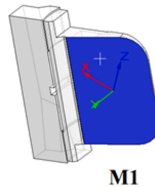
Fig. 8. Orientation of the 1<sup>st</sup> mirror coordinate system.
