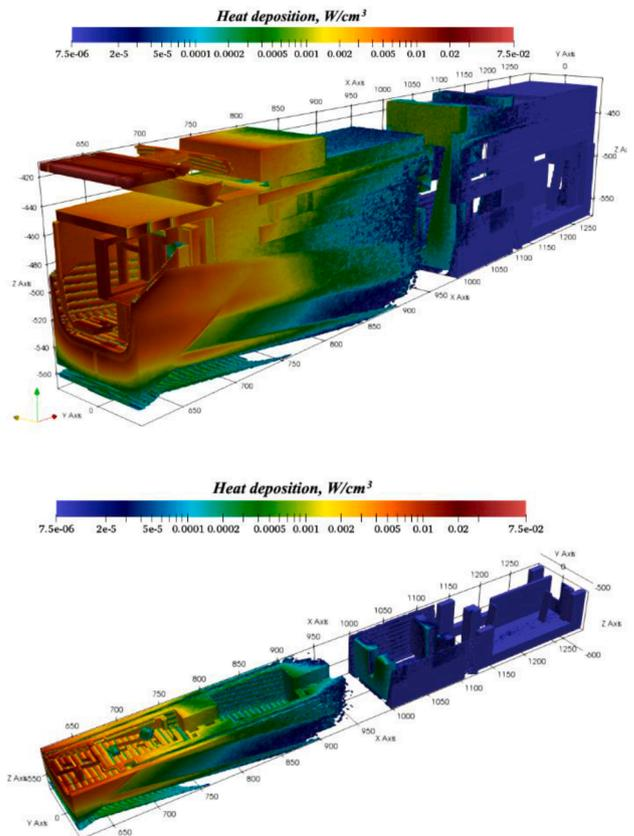
Fig. 3. Nuclear power density in the DTS system (above) and in its horizontal longitudinal cross-section (below), W/cm<sup>3</sup>.
