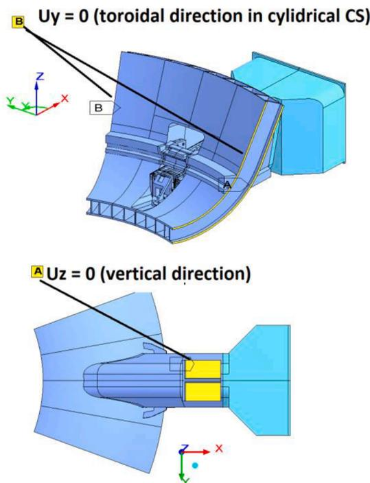
Fig. 7. Structural analysis boundary conditions.
