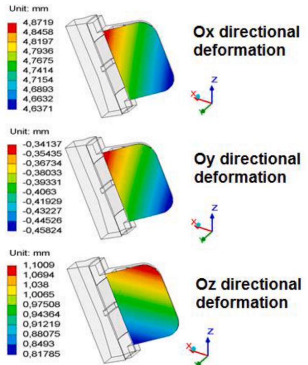
Fig. 9. Deformations of the mirror #1 reflecting surface caused by the normal operation thermal loads, mm.
