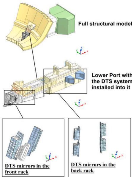
Fig. 1. Full structural model: parts of the vacuum vessel and lower port, DTS system latest design including collecting mirrors.
