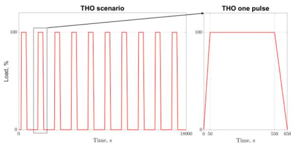
Fig. 2. Loading cycles during normal operation.
