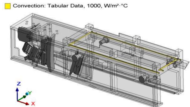
Fig. 4. Cooling water channels (yellow) of the front rack. (For interpretation of the references to color in this figure legend, the reader is referred to the web version of this article.)
